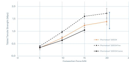
Fig 4: Tablet tensile strength vs Compaction force data of lubricated granules
