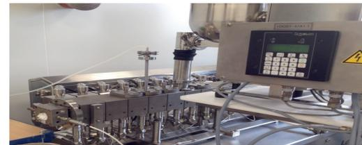
Fig 1: Manufacturing of granules using Leistritz ZSE 18 HPe-VA
