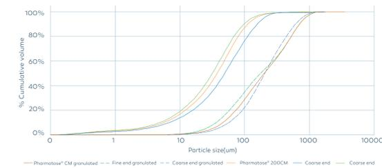
Fig 3: Cumulative PSD graph of Pharmatose® CM along with fine and coarse end
