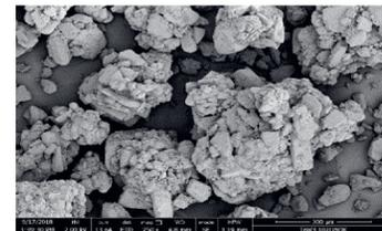
Fig 2: Typical SEM of Pharmatose® CM granules using TSE
