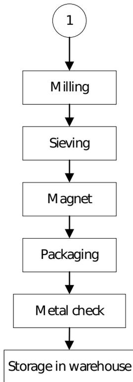
11. The dried lactose is milled to the desired mesh size and passes a 500 µm screen.
