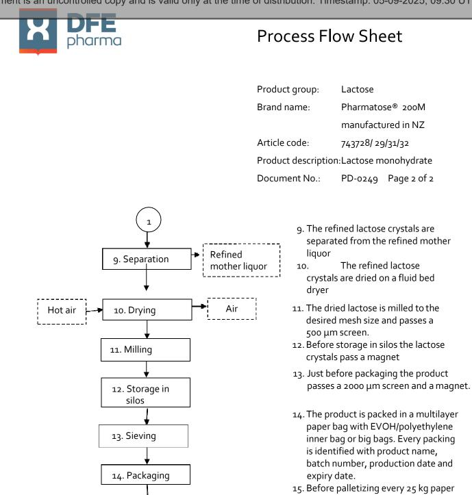
15. Before palletizing every 25 kg paper bag is checked with a metal detector. Sensitivity of the metal detector: Ferrous 1,5 mm, non-ferrous 2,0 mm.
